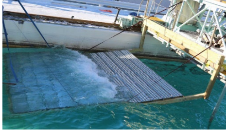
Left: Monitored test wave breaking on the legacy beach in the Ohmsett wave tank.
