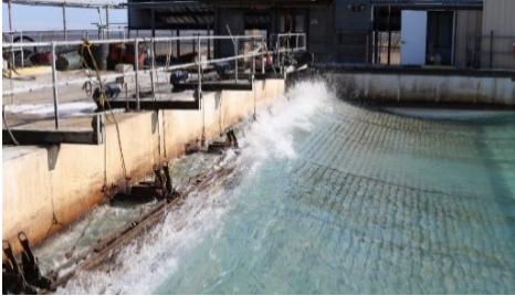
Left: Monitored test wave breaking on the legacy beach in the Ohmsett wave tank.
