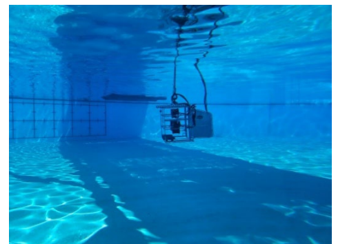
The instrumentation rack is towed through the Ohmsett tank to determine optimal tow speeds.
