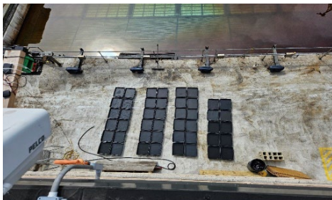
Aerial view of the calibration matrix of known oil thicknesses arrayed on the north deck of the Ohmsett test tank.
