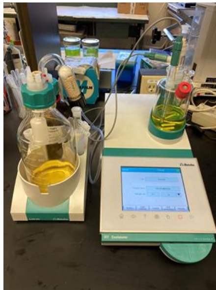
Figure 5 Water content measured with the Metrohm 917 Coulometer
