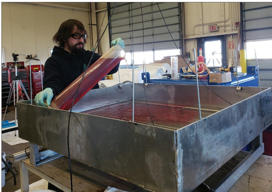
*Ohmsett Technician Allen Cannone prepares the support rack with a known quantity of oil where sorbent samples would be placed. Sorbents were tested for volume of oil recoverable, the rate at which it will adsorb; the amount of water it will adsorb; buoyancy; and the ability for it to be retrieved when fully saturated.*
