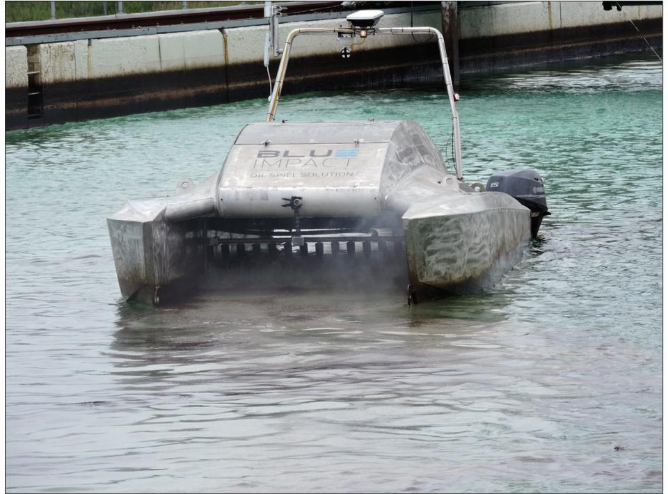
*The Blue Impact mechanical dispersion technology uses high pressure water jets instead of chemicals to disperse oil into the water as tiny droplets.*
