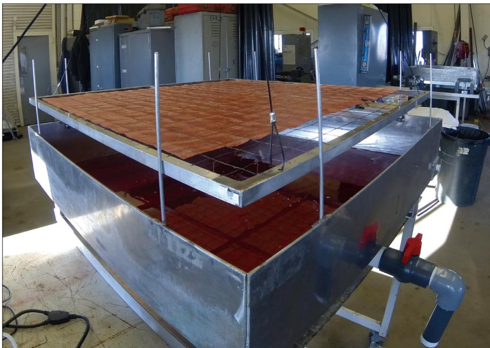
*A support rack was designed to provide consistent handling of the sorbents for minimal contact with the sample. It has the ability to support the sample horizontally and includes a digital weight measurement device.*
