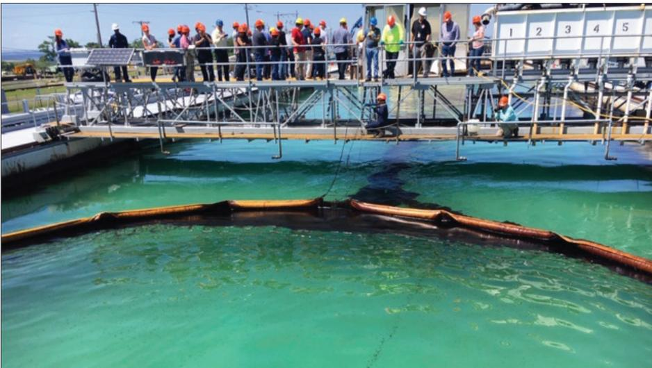
Workshop attendees observe the testing of a new containment boom configuration that directs the oil into a narrow channel of the boom to facilitate in-situ burning without the use of a fire boom.
