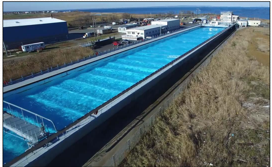
Wave generator and energy damping beach Three equipment and instrumentation tow bridges
