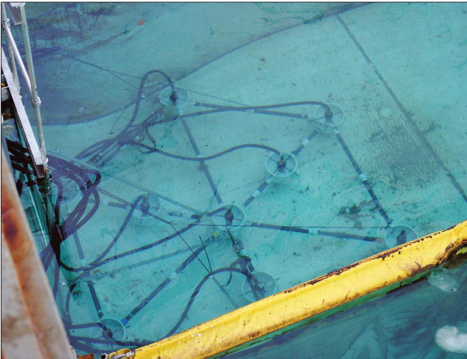
Dynaflow tested a system of microbubble generators (DynaSwirl®) placed beneath a submerged oil plume. The air bubbles adhere to and lift oil droplets and dissolved oil to the surface where they can be removed by traditional oil recovery methods.
