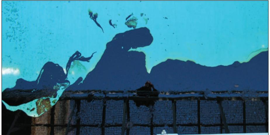
**The combined oil and i-Petrogel adduct was left on the tank surface overnight. The treated oil became a piece of black gel ready to be recovered mechanically.**
