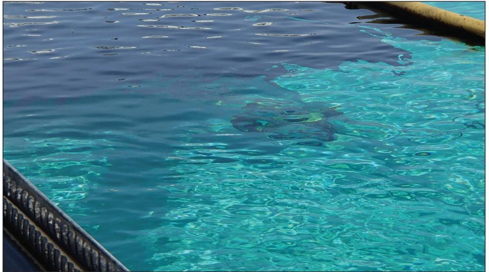
**An ROV, just visible under the oil slick, is fitted with ARA’s acoustic technology to collect measurements of the slick.**
