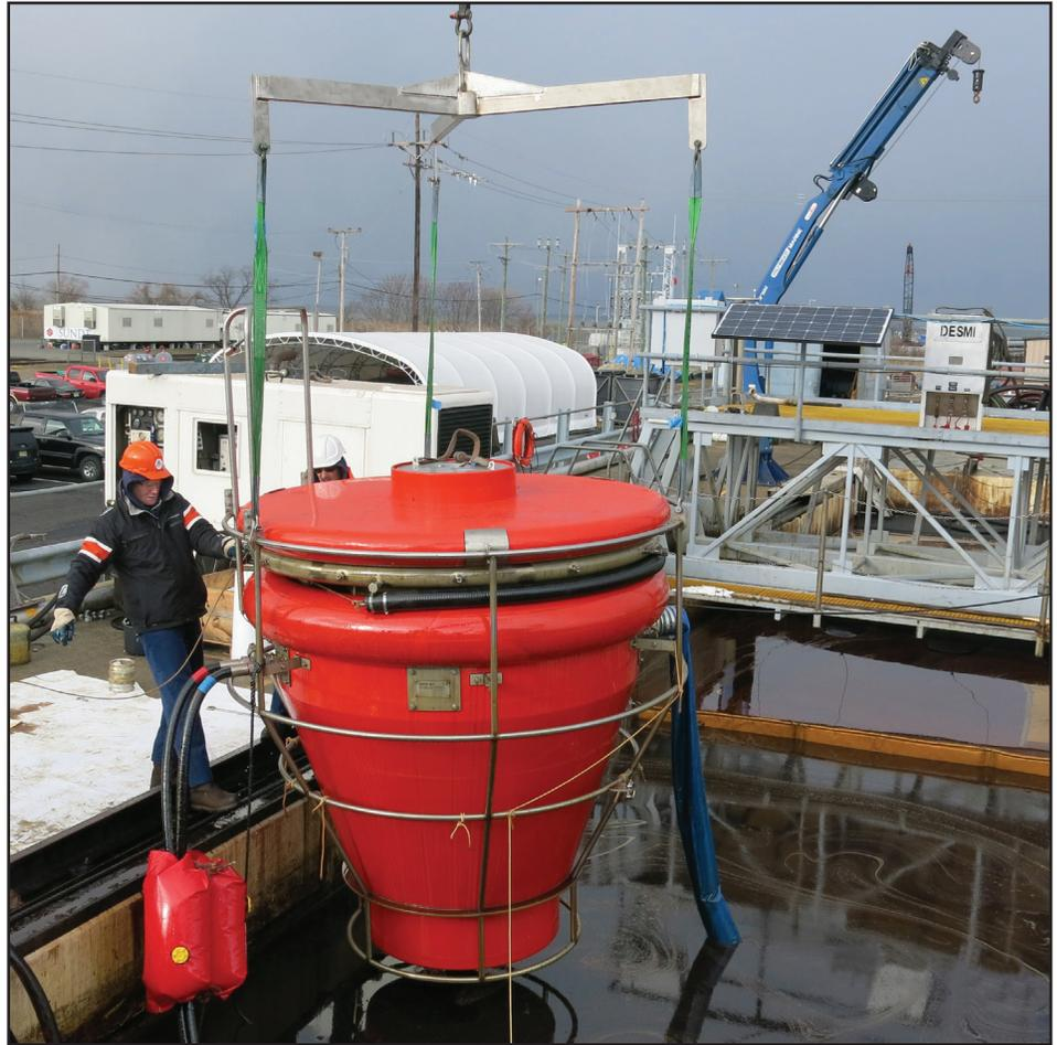
**The FORU stationary skimmer uses an adjustable down draught system that accelerates the water by the inlet perimeter to pull the oil towards the vessel. The system was tested to the ASTM F2709 Standard at Ohmsett during the week of December 8, 2014.**
