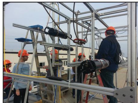
**Instrumentation to locate and analyze a leak is mounted to a frame for testing.**
