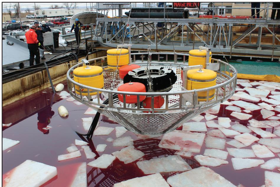
The Desmi Brush skimmer sits inside the ice management system that prevents ice, slush and debris from interfering with the skimmer's ability to pick up oil.
