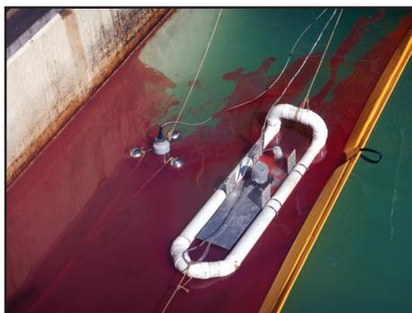
**The Arjay sensors, 2852 HCF on left and 2852-PCD on the sled, travel from clear water into a known oil slick.**
