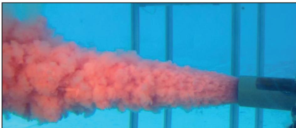
**The Ohmsett staff was able to create subsurface oil flows up to 885 gallons per minute and jet velocities up to 125 feet per second.**
