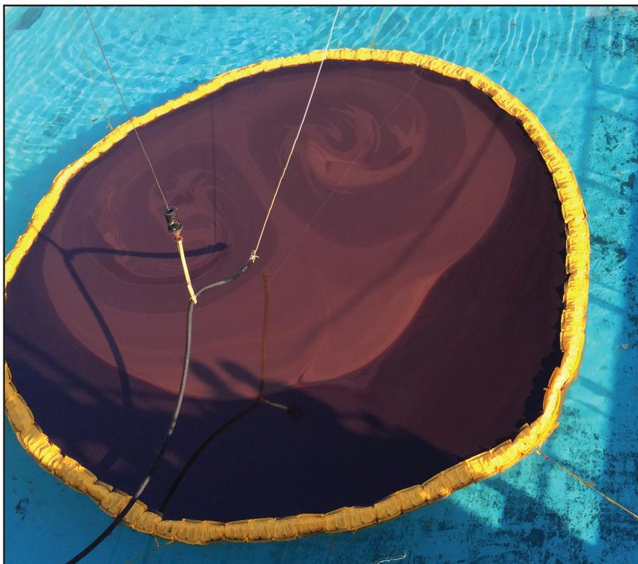
**HARBO modular booms are inflated, and the closed cells are injected with air and sea water. The boom behaves like an integral part of the body of water moving with the currents and waves.**
