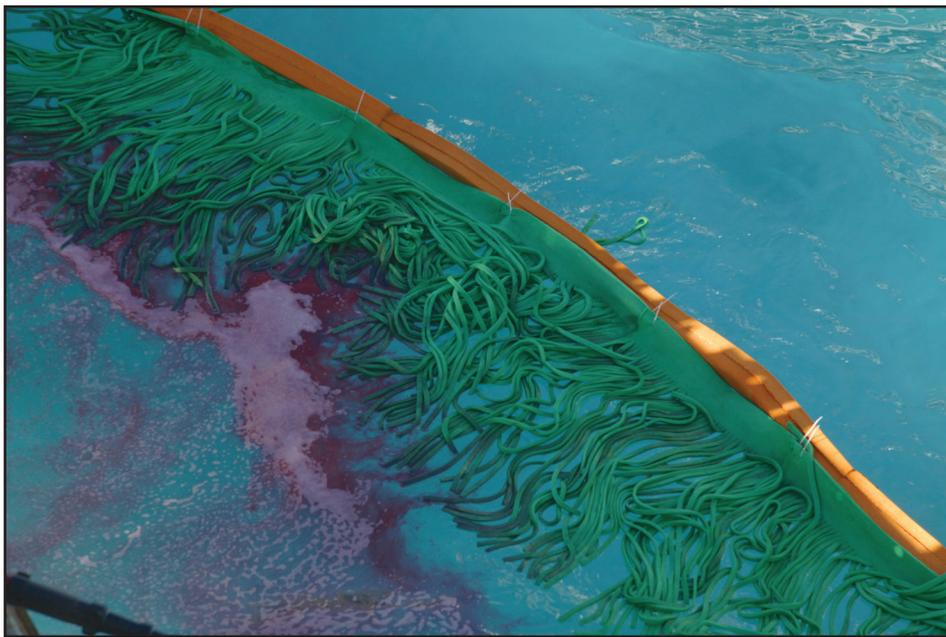
OPFLEX eelgrass was evaluated for its ability to protect a shoreline during a week of testing at Ohmsett.
