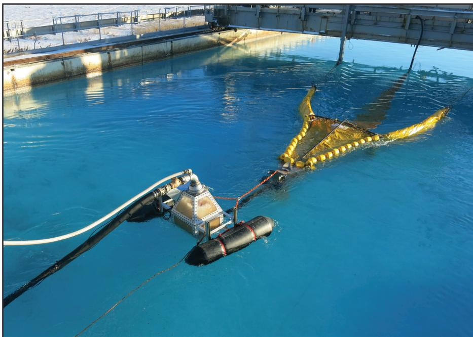
The Vortical Flow Unit of the PPR recovery system creates a natural separation of the oil and water.
