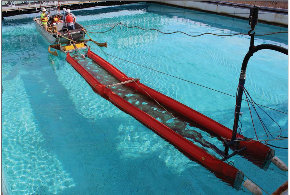
**The autonomous skimmer, outfitted with oil thickness sensors, undergoes performance evaluations in the Ohmsett test basin.**
