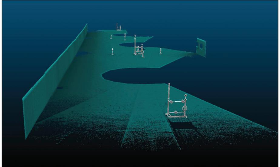
**Targets were placed in precise locations in the Ohmsett test basin. The 3D at Depth underwater laser scanning technology scanned the targets to create the above image.**
