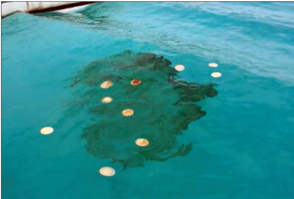
The ocean drifter is designed to move with the ocean swells, currents and waves to track the movement of water and the transport of an oil spill.
