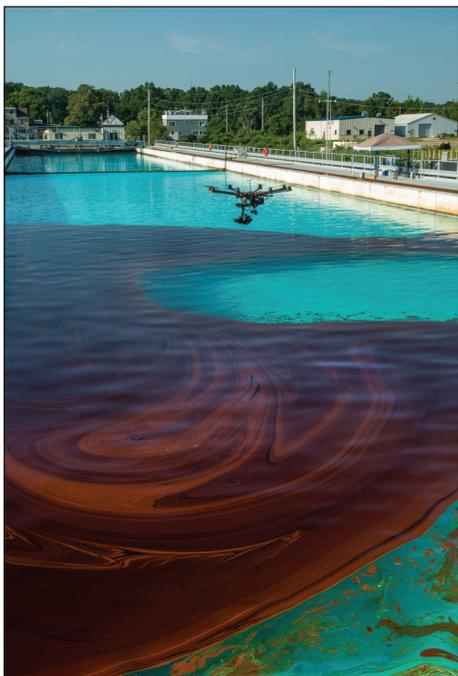
**A rotocraft equipped with a thermal infrared sensor captured images of emulsified oil to validate the sensor's capabilities during the NOAA and BSEE funded remote sensing test.**
