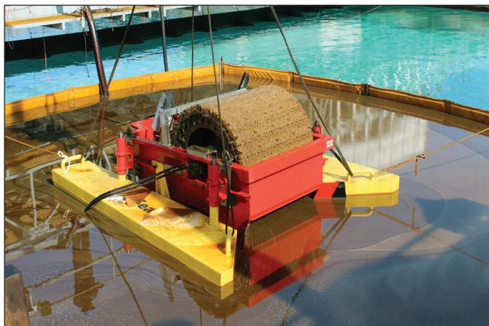
**The SeaHow Offshore skimmer is designed with interchangeable scraper comb plates for varying oil slick viscosities.**
