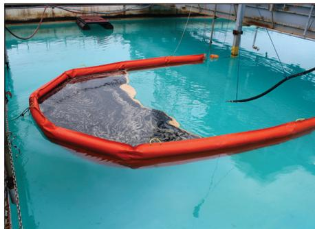
**Dispersant treated oil was placed in the apex of the boom to assess the ability of a boom to contain undispersed oil.**
