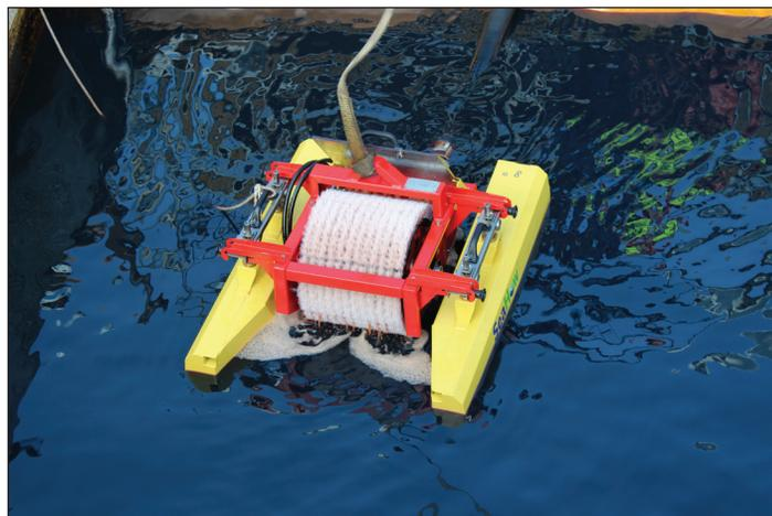
**The MiniSkimmer, a floating skimmer, was evaluated for nameplate recovery rate and recovery efficiency.**
