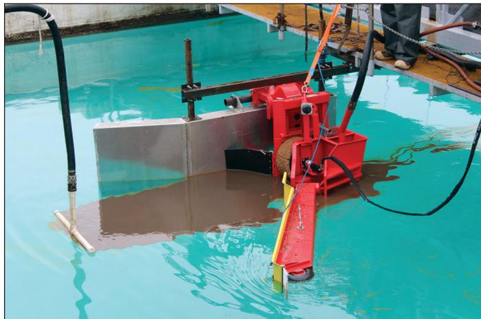
**The MiniBagger is designed with a universal mounting system enabling it to be mounted to small vessels.**
