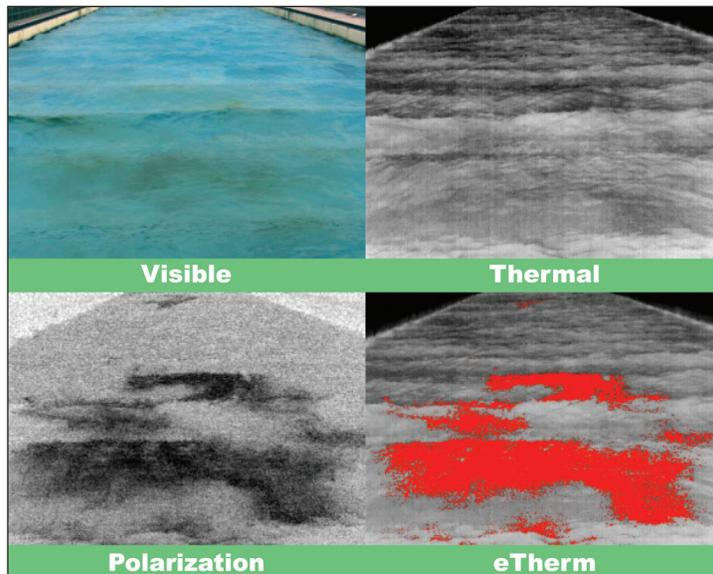
**Thermal, eTherm and polarization comparison data shows the improvement in detection of oil on the waters’ surface using the Pyxis® LWIR.**
