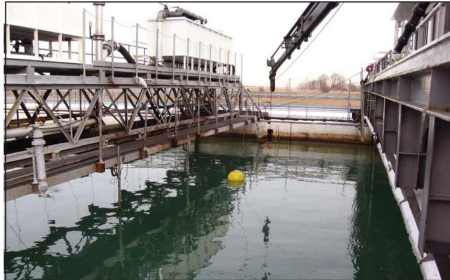
**The Resolute prototype wave energy converter was anchored to the bottom of the Ohmsett wave tank while waves were generated in various configurations to determine certain performance characteristics of the device.**
