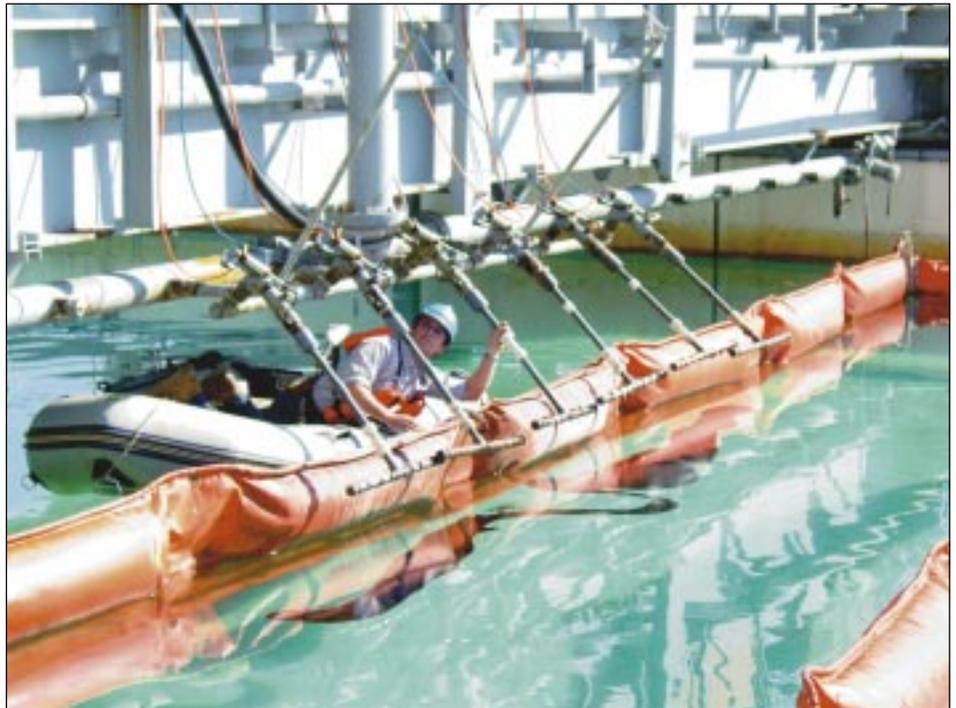
**Ohmsett technician Don Snyder adjusts oil application nozzles in the basin.**
