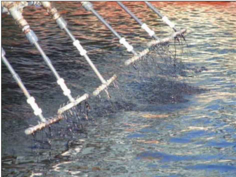
**Oil is applied to the water surface prior to dispersant application.**
