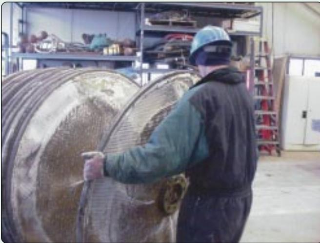
Ohmsett technician John McCall, IV removes the test basin water filter leaves for cleaning.
