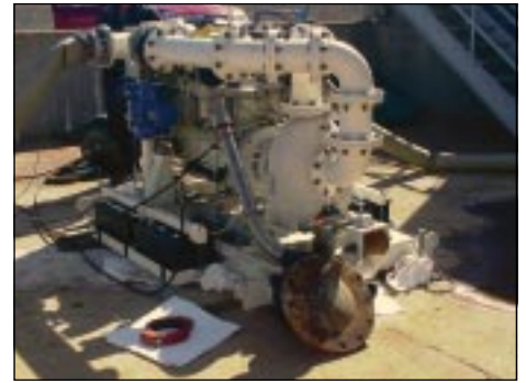
Out of the hull, the Autonomous Marine Booster Pump system is ready to go.
