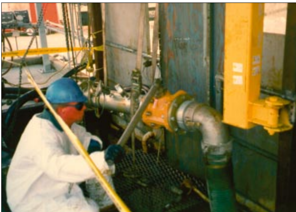
Ohmsett technician Dave Knapp makes adjustments to the discharge valve.
