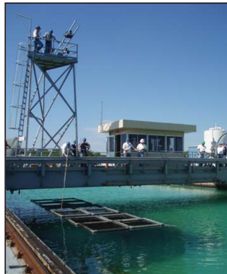
The remote sensing device was mounted on the Main Bridge crow's nest above the oil targets.
