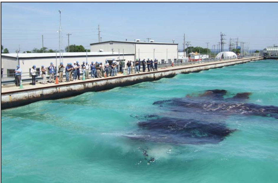
Visitors gather on the deck of the Ohmsett tank to observe the application of dispersant on an oil slick.
