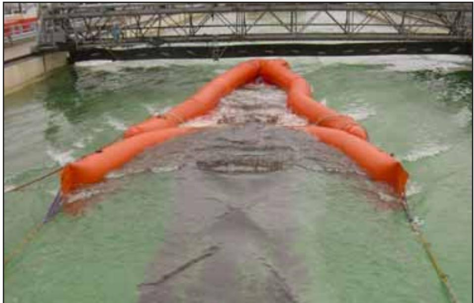
**Slysar Boom undergoing evaluation in the Ohmsett test basin**
