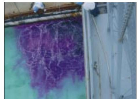
Dye, simulating dispersant, is distributed through the basin water.
