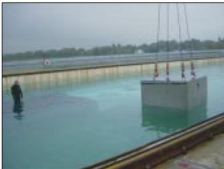
The artificial reef is lowered into the test basin.
