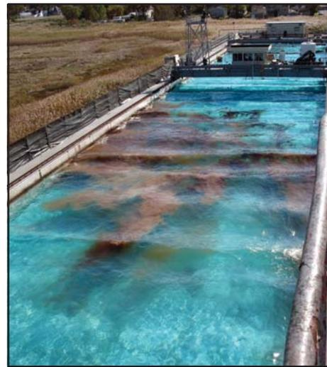
**During the Chemical Herding Agent experiment oil was released on the water and allowed to spread. A herding agent was applied to thicken the slick, after which dispersant was applied.**
