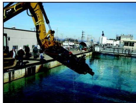
Oil Stop's remote-controlled Sub-Dredge equipped with an EDDY pump, volute, and rotor, can go under, over, or around obstacles to remove sediment or oil.
