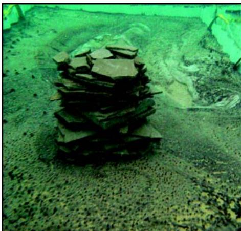
Ohmsett personnel constructed a simulated underwater environment by placing trays containing various sands, rock, stone, dirt, plants, seaweed, and known quantities and thicknesses of oil at the bottom of the test tank.
