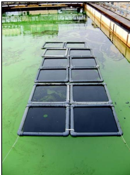
**Oil targets with known quantities of oil were placed in the Ohmsett tank. The remote sensing cameras mounted on the Main Bridge crow's nest were passed over the targets.**
