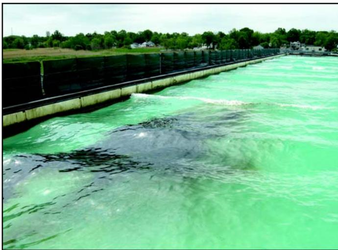
A herding agent was placed on the water surface and oil was gently poured onto the surface. The wave generator was then started, and the slick was allowed to drift until it reached the tank wall or the containment boom.
