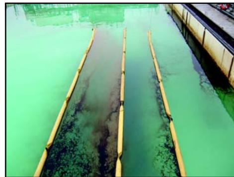
**A set of experiments involved the imaging of fresh and emulsified crude oil before and after it was mixed with a dispersant.**
