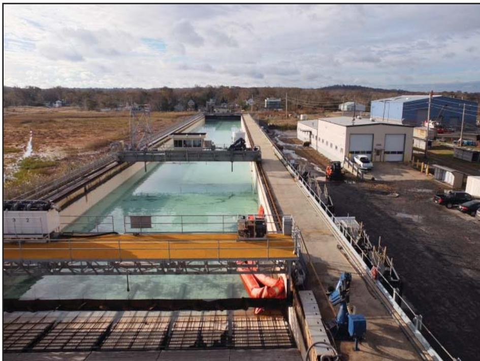
The Ohmsett test tank after the hurricane. The water level in the tank was only two feet; full capacity of the tank is eight feet.
