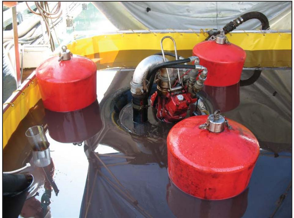
**A draft ASTM skimmer test protocol was tested to resolve issues relating to the significance of slick thickness, oil recovery measurement methods, and minimum tank area required for the test.**
