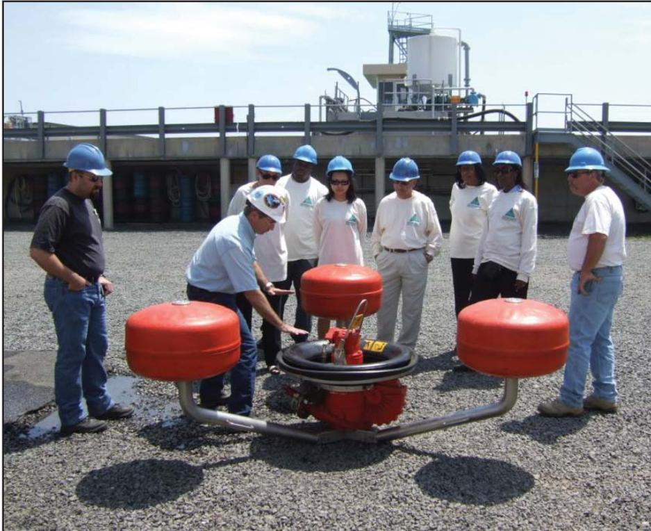
**Joseph Mullin, oceanographer for MMS, explains to the Budget team how a skimmer system is designed to pick up oil during a spill.**
