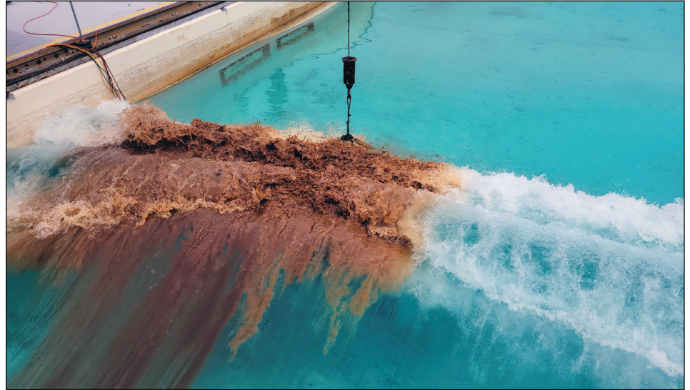
During testing, sensors were mounted to a metal frame. Oil was treated with dispersant and released within the test area. As a breaking wave hit the slick, the instruments measured the effects.
