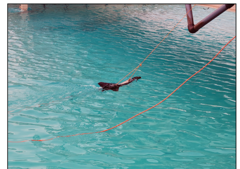
Tethered to the main bridge, the SilCam was towed through the tank during dynamic tests.
