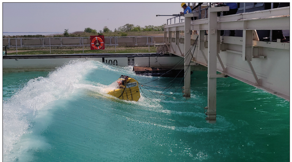
On the Ohmsett tank, OceanEnergy's 1:15 scale floating oscillating water column wave energy converter was studied for operational and structural performance.
