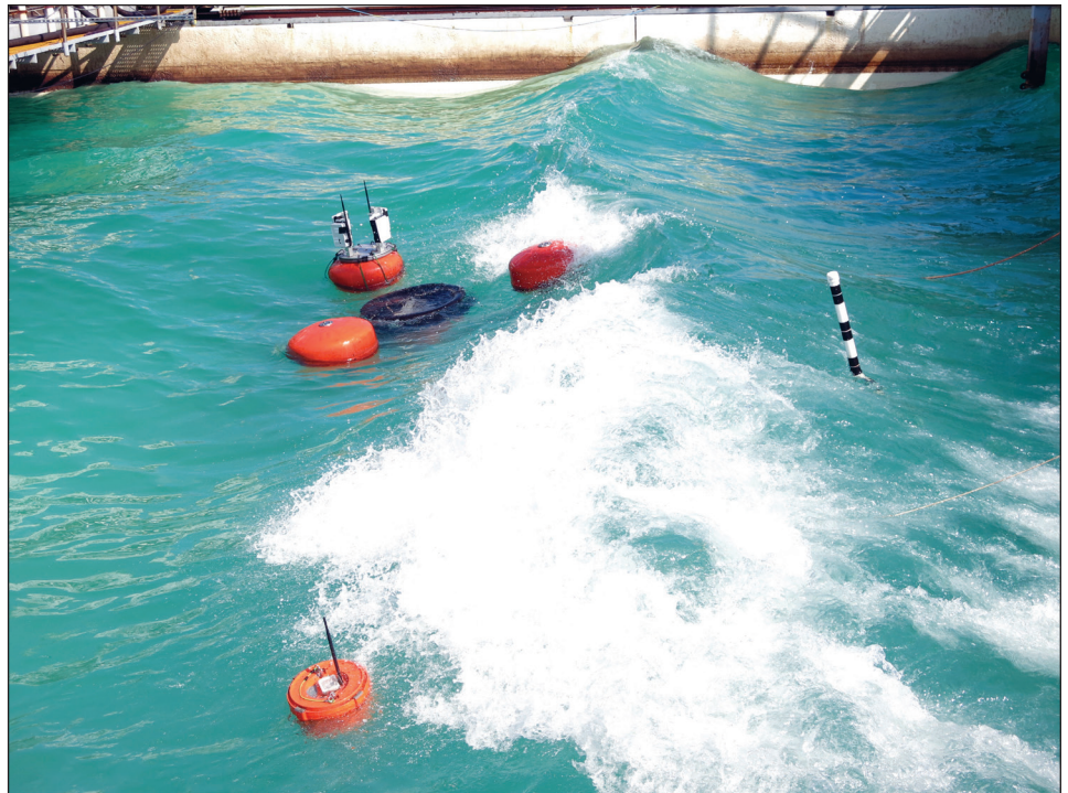
A tagging system equipped with a wave characterization module is mounted to a skimmer to track the skimmer location and wave conditions during spill response operations.
