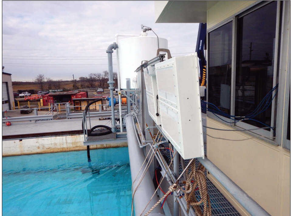
The ISPAS Oil Spill Detection (OSD) radar was evaluated at Ohmsett. Mounted to the main bridge, the radar was tested for its ability to detect an oil spill in calm water and waves.
