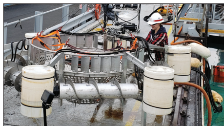
The Active Ice Management System (AIMS) is designed to redirect the floating ice away from the system so oil can be easily drawn to the skimmer for recovery.
