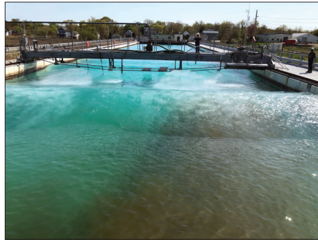
Dispersant was applied to an oil slick using a hand-held pressurized nozzle system. The treated slick was then subjected to waves programmed to break at the location of the slick in the Ohmsett test tank.
