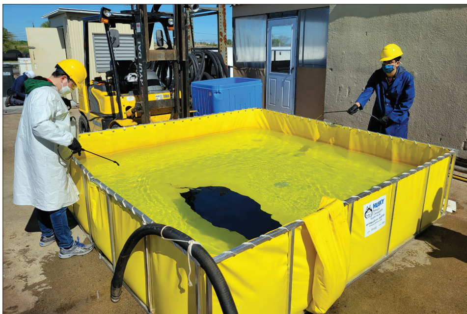
LSU conducted a series of scaled-up experiments at the Ohmsett facility to verify laboratory scale data related to the interaction of lignin nanoparticles with oil slicks on water.
