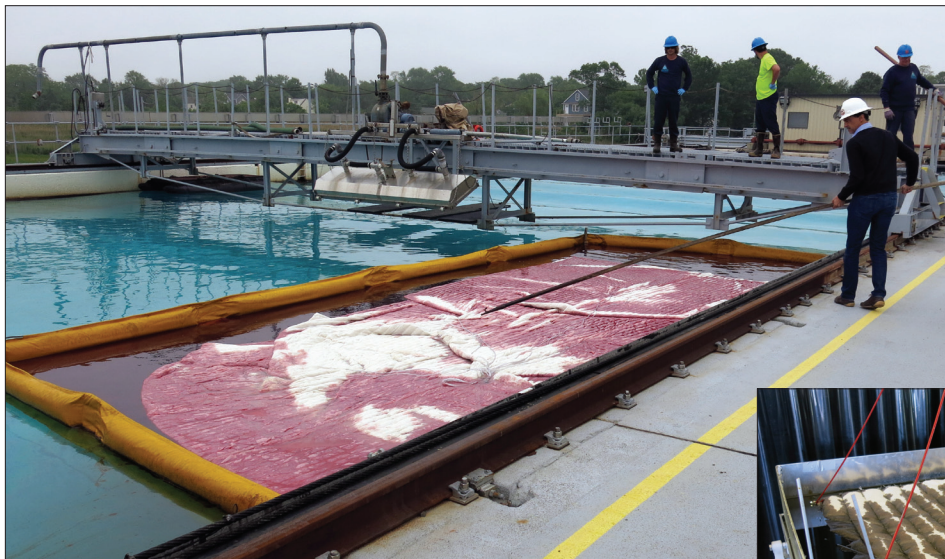
Full scale tests were performed in a boomed area in the basin to demonstrate the deployment of large scale organic oleophilic spill mats onto a controlled spill scenario.
