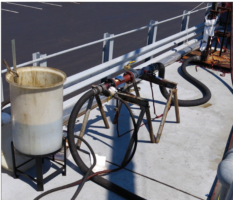
Battelle Memorial Institute developed a recovery efficiency sensor that could be installed in-line between the skimmer and the storage tank that measures, in real time, the amount of oil that is being recovered.
