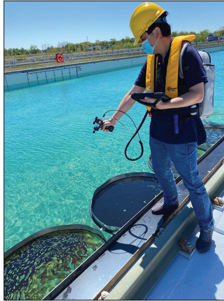
Dr. Chuanmin Hu from the University of South Florida collected data to support estimates of surface slick thickness from the test rings using a radiometer.
