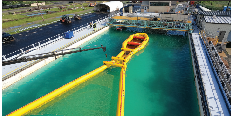
The NOFI Current Buster 4 runs through tests with three types of oil to validate and verify its ability to collect oil at 4.4 knots with and without waves.
