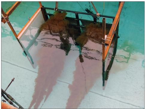
Argonne National Lab's Oleo Sponge prototype is a reusable chemically treated polyurethane foam to adsorb submerged oil. Multiple Oleo Sponge panels were attached to a metal frame and mounted to the auxiliary bridge where it encountered suspended oil plumes.
