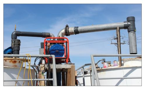
The Zelda II HVLS pump can be powered by a hydraulic motor or by a hand crank. The low operational speed reduces wear, heat and the possibility of cavitation and emulsification.
