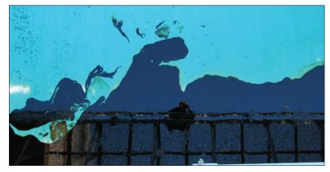
The combined oil and i-Petrogel adduct was left on the tank surface overnight. The treated oil became a piece of black gel ready to be recovered mechanically.
