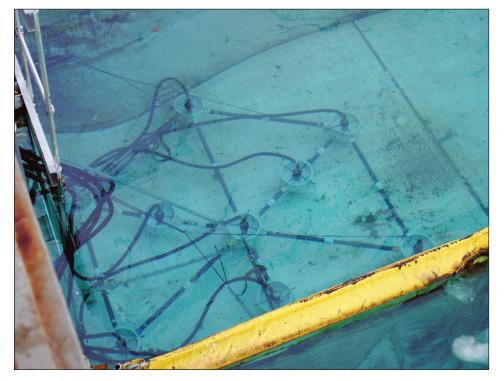
Dynaflow tested a system of microbubble generators (DynaSwirl<sup>®</sup>) placed beneath a submerged oil plume. The air bubbles adhere to and lift oil droplets and dissolved oil to the surface where they can be removed by traditional oil recovery methods.
