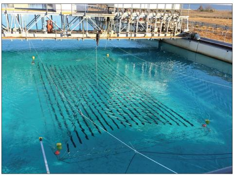
This prototype macroalgae culture system will allow kelp to grow in the open ocean to help improve the ecosystem by absorbing CO, and excess nutrients.
